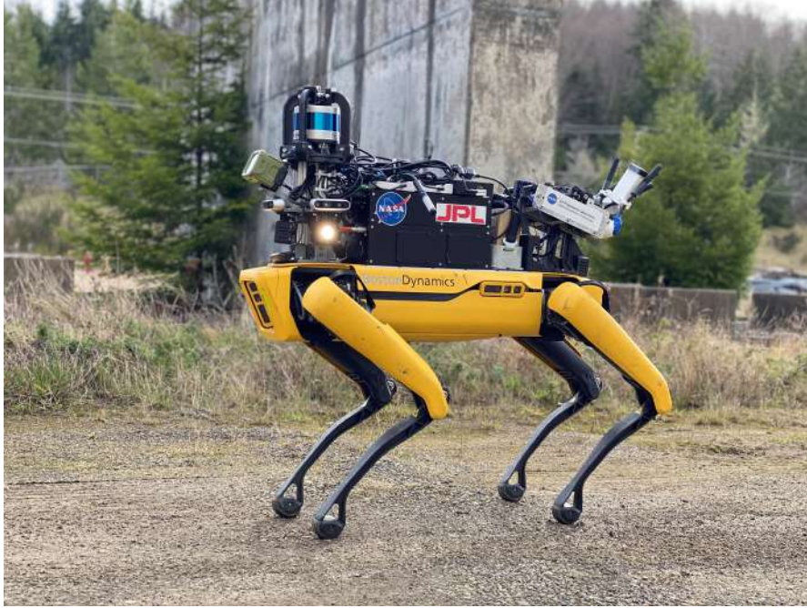
Figure 1.1: Boston Dynamics Spot integrated with the NeBula autonomy stack (“Au-Spot”): Spot base with the NeBula Sensor Package (NSP) and the NeBula Power and Computing Core (NPCC). The platform was deployed in the DARPA Subterranean Challenge and demonstrates building-scale autonomy on a legged robot (Agha et al. , 2021; Bouman et al. , 2020).
