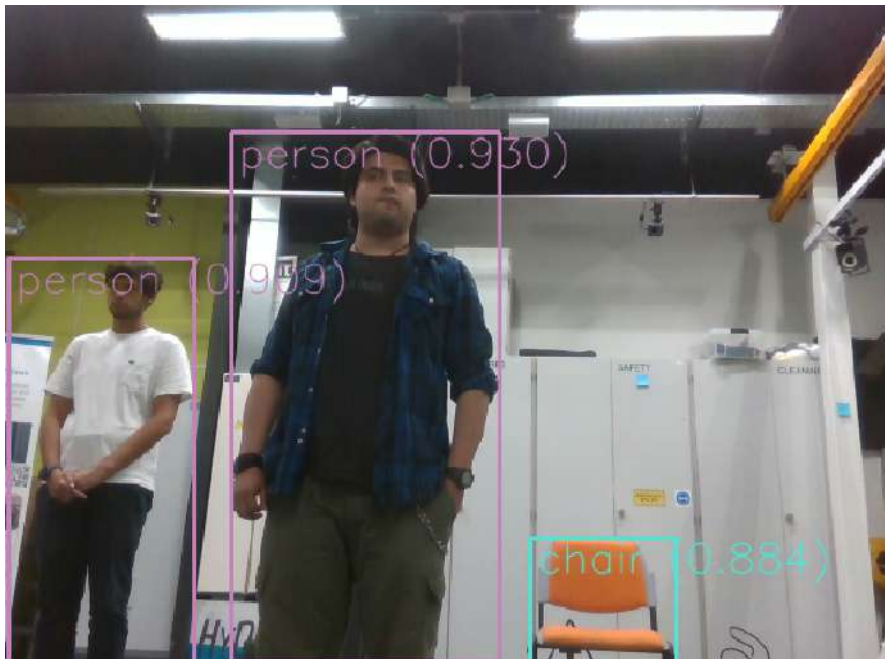
Figure 4.4: Example YOLO output from the robot’s RGB camera during the DLS lab experiment. The detector runs on the D435 colour stream and overlays class labels and confidence scores, here identifying two person instances and one chair . This is the same scene used for the semantic mapping experiment in Figures 4.5 and 4.6.
